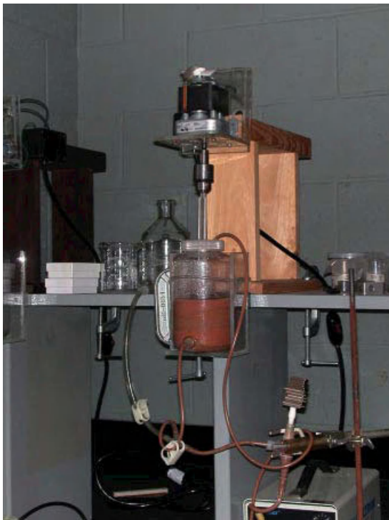
Plate 27 (Figure 9.3) Example of a magnetic extraction set-up. Slurry from a pulverized red bed was centrifuged to produce the red-colored material in the device. Hematite particles were extracted and their individual particle anisotropy was measured (Kodama 2009).
